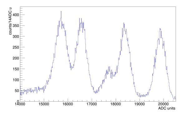
Figure 4.2: Energy spectrum for a sample strip from the  $^{228}$ Th calibration run. Note that the gain from the preamplifier was such that the higher-energy  $\alpha$  particle at 8.785 MeV was not visible.
