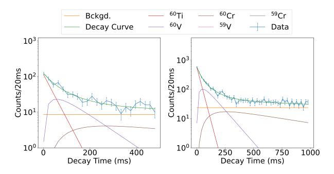
Figure A.7: Decay curves for the  $^{60}$ Ti isotopes for both the BCS-NERO (left) and SuN (right) portions. Legends are identical for both.
