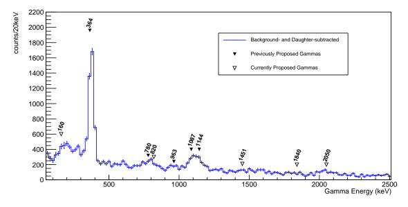
Figure C.5: Final, background- and daughter-subtracted SS for the  $^{57}$ Sc decay. Closed triangles show the previously identified  $\gamma$ -rays [19], while the open triangles indicate proposed  $\gamma$ -rays from this work.
