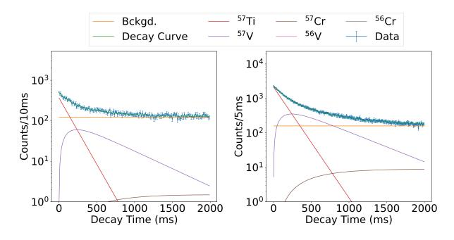
Figure A.4: Decay curves for the  $^{57}$ Ti isotopes for both the BCS-NERO (left) and SuN (right) portions. Legends are identical for both. In this 500 ms window, only the parent  $^{57}$ Ti and daughter  $^{57}$ V decays appear in appreciable amounts.
