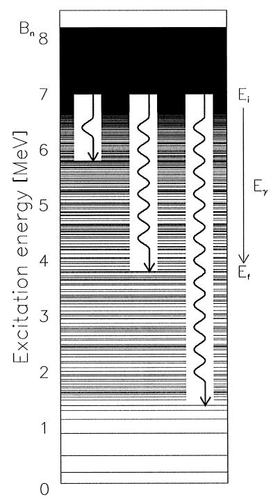
Figure 3.3: Generic example of the increase in the nuclear level density from discrete states (roughly  $0-1.5\,\mathrm{MeV}$ ) to a quasi-continuum (roughly  $>1.5\,\mathrm{MeV}$ ). Figure is reproduced from [45].
