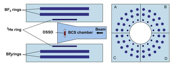
Figure 2.4: A schematic of the BCS inside the NERO array. Note that NERO is arranged such that the BCS DSSD is at the center of the NERO detectors to maximize neutron detection efficiency. Figure reproduced from [27].
