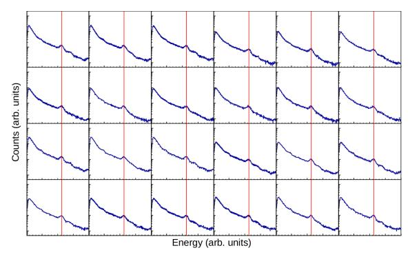
Figure 4.9: Histograms of the individual PMTs in SuN for a background run. A vertical line is drawn through the  $^{40}$ K  $\gamma$ -ray peak to which all of the PMTs are gain matched.
