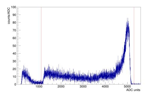
Figure 4.7: Sample spectra for the NERO <sup>3</sup>He neutron counting tubes. Visible is the low energy noise peak, along with the designated upper and lower limits (red vertical lines) of a neutron signal for these tubes. Only signals within the red bounds were considered neutron events, and the bounds are set for each tube individually.
