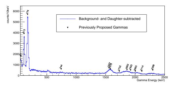
Figure B.6: Final, background- and daughter-subtracted SS for the  $^{57}$ Ti decay. Note the two levels from  $^{57}$ V are now removed. Closed triangles show the previously identified  $\gamma$ -rays [18], while the open triangles indicate proposed levels from this work. The peak at 511 keV is due to electron pair production.
