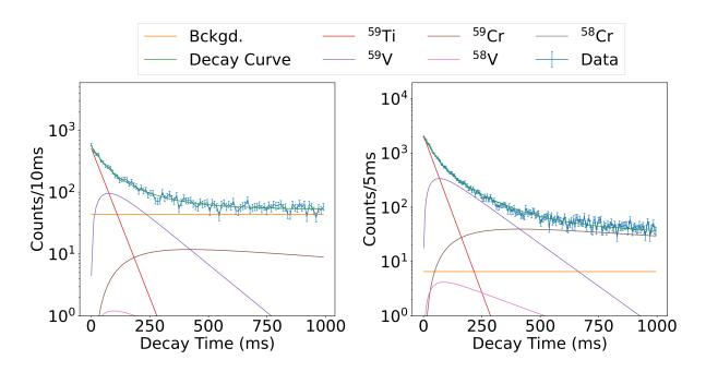
Figure A.6: Decay curves for the <sup>59</sup>Ti isotopes for both the BCS-NERO (left) and SuN (right) portions. Legends are identical for both.
