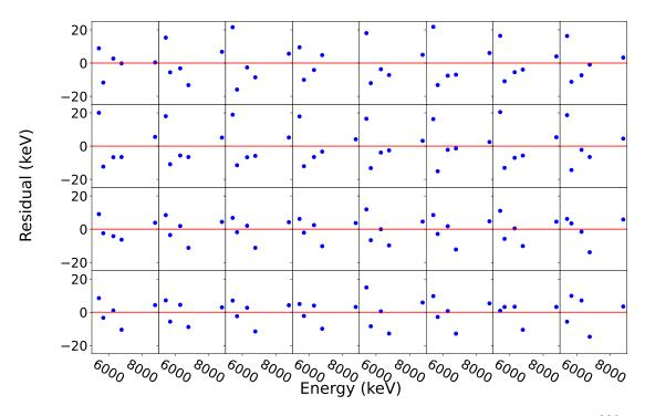
Figure 4.12: Residuals of the linear calibration of the SuN DSSD strips to the  $^{228}$ Th source data.
