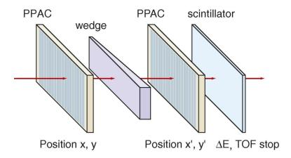
Figure 2.2: Schematic of the wedge-shaped energy degrader in the A1900 separator [29, 30] at the Image 2 position. Also seen here is the scintillator, which acted as the stop gate on the time-of-flight calculation for particle identification. Figure reproduced from [29].
