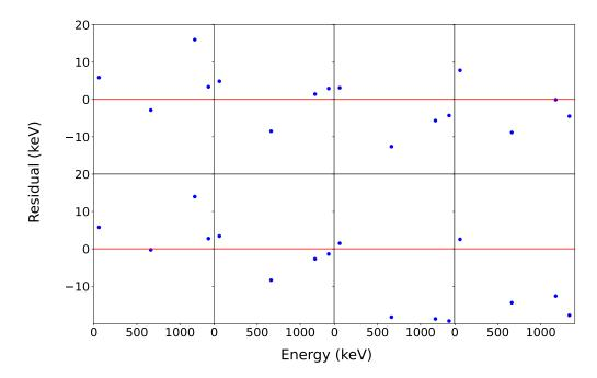
Figure 4.11: Residuals of the post-experiment calibration using the pre-experiment linear fit of the eight SuN segments to the calibration  $\gamma$ -rays from  $^{241}\mathrm{Am}$ ,  $^{137}\mathrm{Cs}$  and  $^{60}\mathrm{Co}$ .
