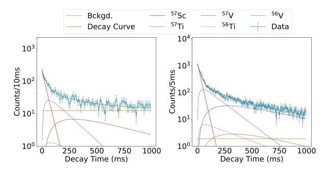
Figure A.3: Decay curves for the  $^{57}$ Sc isotopes for both the BCS-NERO (left) and SuN (right) portions. Legends are identical for both.
