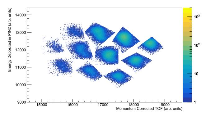
Figure 4.15: Particle ID ( $\delta$ E-TOF) plots for the BCS-NERO portion, cut on isotopes of interest. From left to right, top to bottom:  $^{62}$ V,  $^{61}$ V,  $^{60}$ V,  $^{59}$ V,  $^{60}$ Ti,  $^{59}$ Ti,  $^{58}$ Ti,  $^{57}$ Ti,  $^{57}$ Sc,  $^{56}$ Sc,  $^{55}$ Sc.
