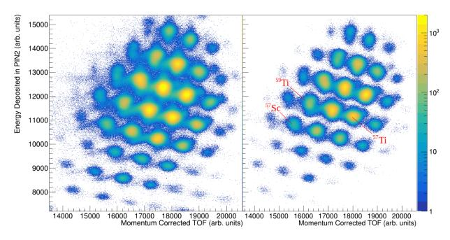
Figure 4.16: Particle ID ( $\delta$ E-TOF) plots for the SuN portion. Left shows all the beam particles that passed through the upstream PINs, right is the same but cut to only the particles successfully implanted in the DSSD. The visible "shadow" between some isotopes is due to trigger thresholds in the I2 scintillator. Particle cuts are applied in order to reduce the contribution from these events.
