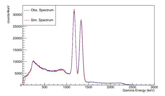
Figure 3.1: Histograms of the SuN SS for an observed (blue) and simulated (red)  $^{60}$ Co source. Both are filtered to only include events with multiplicity  $\geq 2$ .
