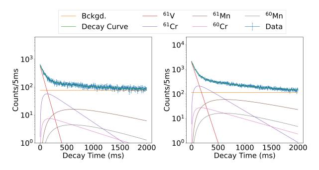
Figure A.10: Decay curves for the  $^{61}$ V isotopes for both the BCS-NERO (left) and SuN (right) portions. Legends are identical for both.
