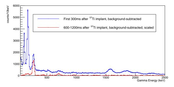
Figure B.5: Background-subtracted SS for  $t < 300\,\mathrm{ms}$  after implantation (blue) and the region  $600 < t < 1200\,\mathrm{ms}$  (red) for the  $^{57}\mathrm{Ti}$  decay. Note the two  $\gamma$ -rays at  $268\,\mathrm{keV}$  and  $692\,\mathrm{keV}$  which are due to the  $\beta$ -daughter decay of  $^{57}\mathrm{V}$ .
