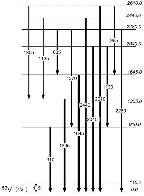
Figure D.1:  $^{59}{\rm V}$  level scheme for the  $\beta$  decay of  $^{59}{\rm Ti}$  to  $^{59}{\rm V}.$
