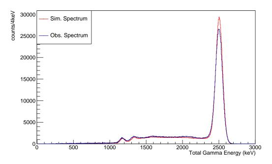
Figure 3.2: Histograms of the SuN TAS for an observed (blue) and simulated (red)  $^{60}$ Co source. Both are filtered to only include events with multiplicity  $\geq 2$ .
