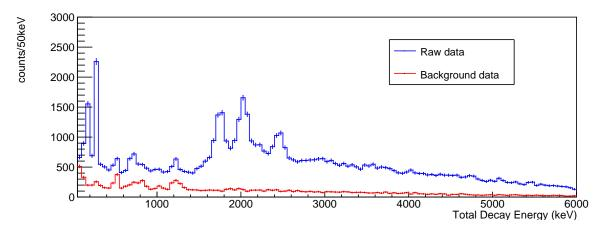
Figure B.2: Raw, forward-correlated TAS (blue) and reverse-correlated background TAS (red) for the  $^{57}\mathrm{Ti}$  decay. Both are cut to only include decays in the first 300 ms after implantation.
