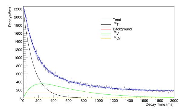
Figure 4.18: Decay time plot including parent, background, and all daughter decay curves from  $^{57}$ Ti correlated decays. Neutron-daughter decays are not included here as the  $P_{\rm n}$  was determined to be negligible.
