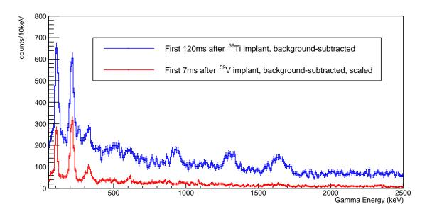
Figure D.4: Reverse-time background subtracted SS of the correlated decays within the first  $120 \,\mathrm{ms}$  following  $^{59}\mathrm{Ti}$  implants (blue), with the reverse-time background subtracted and scaled SS of the correlated decays within the first  $7 \,\mathrm{ms}$  following  $^{59}\mathrm{V}$  implants (red).
