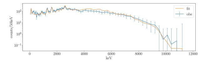
Figure D.7: TAS for the  $^{59}$ Ti decay, for the entire energy spectrum to the Q-value.
