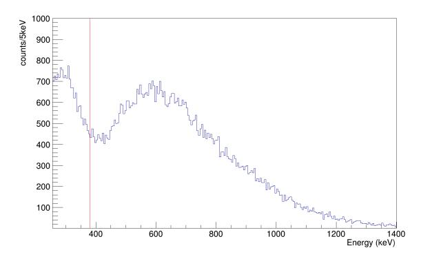
Figure 4.5: Energy spectrum for a sample strip from the  $^{90}$ Sr calibration run. The software threshold for the sample strip is shown by the red line.
