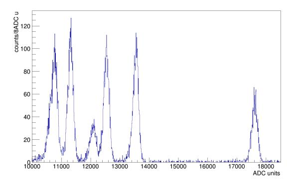
Figure 4.13: Energy spectrum for a sample strip from the <sup>228</sup>Th calibration run.
