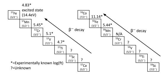
Figure 1.4: State of ground state spins and ground state to ground state transitions for A = 57,59 mass chains. These run from the neutron-rich nuclei expected to contribute to Urca cooling back to stability.
