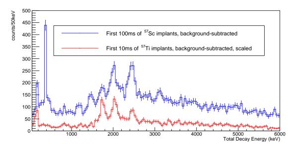
Figure C.2: Reverse-time background subtracted TAS of the correlated decays within the first  $100\,\mathrm{ms}$  following  $^{57}\mathrm{Sc}$  implants (blue), with the reverse-time background subtracted and scaled TAS of the correlated decays within the first  $10\,\mathrm{ms}$  following  $^{57}\mathrm{Ti}$  implants (red).
