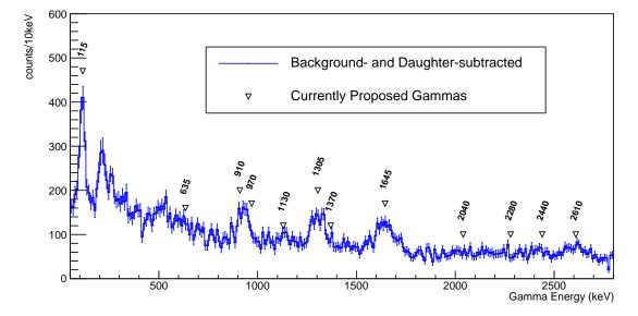
Figure D.5: Final, background- and daughter-subtracted SS for the  $^{59}$ Ti decay. Open triangles indicate proposed levels from this work. As with  $^{57}$ Ti, the small peak at 511 keV is due to pair production in the detector from high-energy  $\gamma$ -rays. The peak around 210 keV is not labeled as no coincidences were established, nor is a specific TAS level clear. It is likely due to incomplete daughter subtraction.
