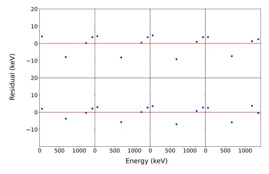
Figure 4.10: Residuals of the linear fit of the eight SuN segments to the calibration  $\gamma$ -rays from  $^{241}{\rm Am},~^{137}{\rm Cs},$  and  $^{60}{\rm Co}.$
