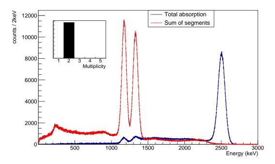
Figure 2.8: Same as Fig. 2.7 but now only including events with an exact multiplicity of two segments. The inset multiplicity distribution (black) demonstrates this cut.
