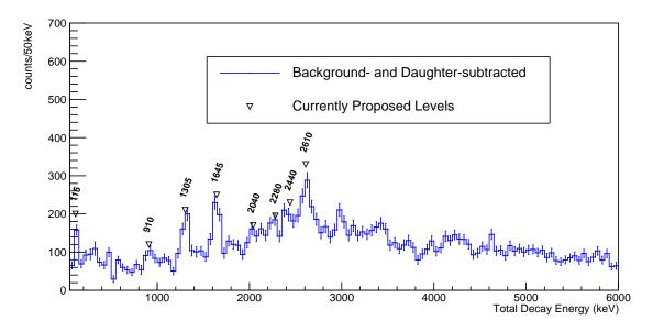
Figure D.3: Final, background- and daughter-subtracted TAS for the  $^{59}{\rm Ti}$  decay. Open triangles indicate proposed levels from this work.
