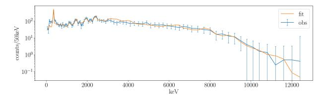
Figure C.7: TAS for the  $^{57}$ Sc decay, for the entire energy spectrum to the Q-value.
