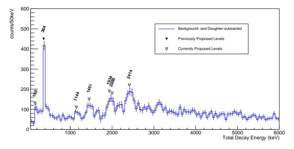
Figure C.3: Final, background- and daughter-subtracted TAS for the <sup>57</sup>Sc decay. Closed triangles show the previously proposed levels [19], while the open triangles indicate proposed levels from this work.
