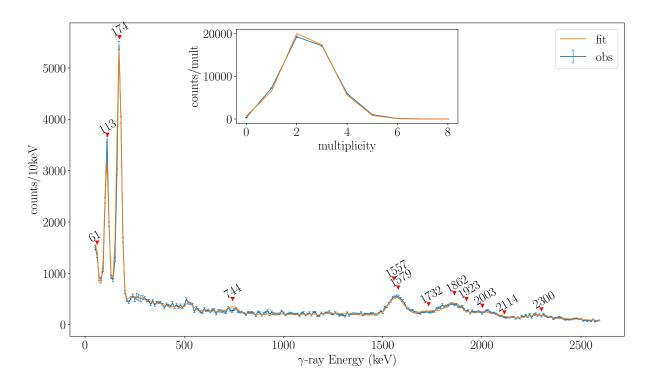
Figure B.9: SS for the  $^{57}\mathrm{Ti}$  decay, the multiplicity fit is inset.
