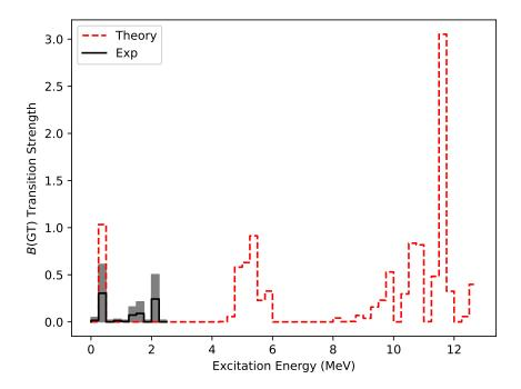
Figure 6.2: Comparison of QRPA predicted (dashed red) and experimentally observed (black, with gray shaded errors) B(GT) transition strengths for the decay of  $^{57}$ Sc to  $^{57}$ Ti.  $S_{\rm n}$  of  $^{57}$ Ti is at 2.67 MeV.
