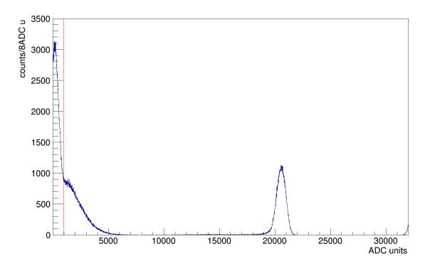
Figure 4.1: Spectra of a sample strip from the  $^{241}$ Am and  $^{90}$ Sr joint source run. Visible is the noise peak below the threshold (red line) at  $\sim 1950$  ADC units which transitions into the  $^{90}$ Sr electron  $\beta$ -decay spectrum. The  $^{241}$ Am  $\alpha$ -decay at  $\sim 20000$  ADC units is used to gain-match the energies of each SSSD strip.
