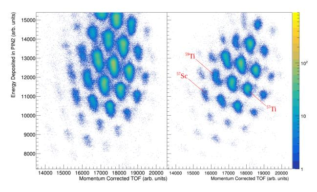
Figure 4.14: Particle ID ( $\delta$ E-TOF) plots for the BCS-NERO portion. Left shows all the beam particles that passed through the upstream PINs, right is the same but cut to only the particles successfully implanted in the DSSD.
