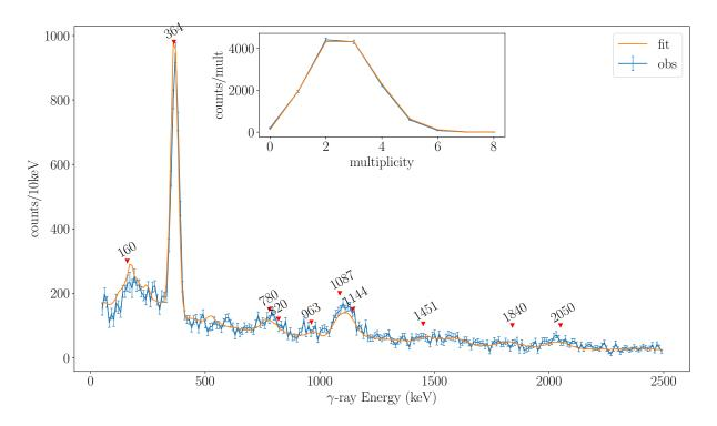
Figure C.8: SS for the  $^{57}$ Sc decay, the multiplicity fit is inset.
