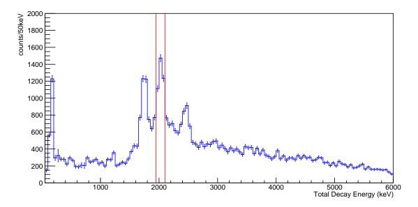
Figure 3.4: Background- and daughter-subtracted TAS for  $^{57}$ Ti correlated decays. Red lines indicate the gates applied to select the level at 2036 keV. The black dashed line shows the cutoff,  $E_{\rm crit}=2550\,{\rm keV}$ , at which the discrete level region ends and the quasi-continuum begins.
