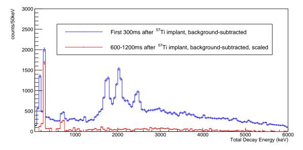
Figure B.3: Background-subtracted TAS for  $t < 300 \,\mathrm{ms}$  after implantation (blue) and the region  $600 < t < 1200 \,\mathrm{ms}$  (red) for the  $^{57}\mathrm{Ti}$  decay. Note the two levels at  $268 \,\mathrm{keV}$  and  $692 \,\mathrm{keV}$  which are due to the  $\beta$ -daughter decay of  $^{57}\mathrm{V}$ .
