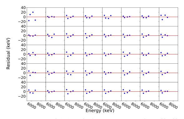
Figure 4.3: Residuals of the linear fit of the back side strips of the BCS DSSD to the calibration  $\alpha$  particles from <sup>228</sup>Th decay. Note that the gain from the preamplifier was such that none of the spectra included the higher-energy  $\alpha$  particle at 8.785 MeV.
