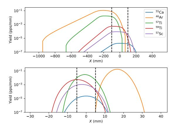
Figure 2.3: LISE<sup>++</sup> simulated yield vs. X at Image 1 (top) and at the focal plane (bottom) in the A1900. The dashed black lines indicate the slits selecting on X position at Image 1 ( $\pm 100\,\mathrm{mm}$ ), and at the focal plane ( $\pm 5\,\mathrm{mm}$ ). Only the particles of interest and the sample contaminant  $^{46}\mathrm{Ar}$  are shown.
