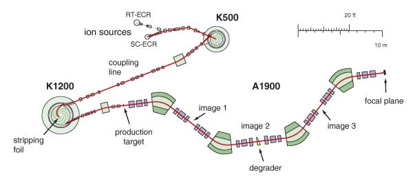
Figure 2.1: Schematic of the CCF and A1900 at the NSCL, figure reproduced from [29]. Particularly of note is the wedge degrader at Image 2, which was used to further separate beam components by momentum. Immediately downstream of the degrader is a scintillator (not pictured) with two photomultiplier tubes used as a time-of-flight trigger for particle identification [29, 30].
