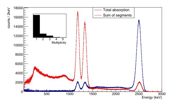
Figure 2.7: Overlaid comparison of the two main spectra observed by SuN in the  $^{60}$ Co decay: the sum of individual segments (red), and the total absorption (blue). Visible are the two separate individual  $\gamma$ -ray peaks in the sum of segments, as well as the clear sum peak in the total absorption. Inset is the multiplicity distribution in black, from 1 to 5 distinct segments.
