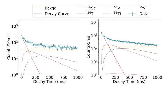
Figure A.2: Decay curves for the  $^{56}$ Sc isotopes for both the BCS-NERO (left) and SuN (right) portions. Legends are identical for both.
