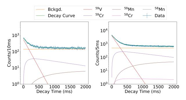
Figure A.8: Decay curves for the  $^{59}$ V isotopes for both the BCS-NERO (left) and SuN (right) portions. Legends are identical for both.
