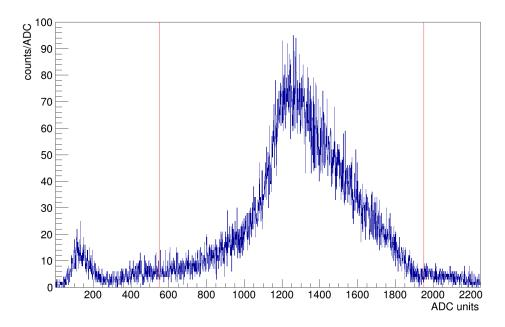
Figure 4.8: Sample spectra for the NERO BF<sub>3</sub> neutron counting tubes. Visible is the low energy noise peak, along with the designated upper and lower limits (red vertical lines) of a neutron signal for these tubes. Only signals within the red bounds were considered neutron events, and the bounds are set for each tube individually.
