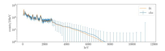
Figure D.9: Log-scaled SS for the  $^{59}\mathrm{Ti}$  decay, including higher energy  $\gamma$ -rays.
