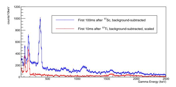
Figure C.4: Reverse-time background subtracted SS of the correlated decays within the first  $100\,\mathrm{ms}$  following  $^{57}\mathrm{Sc}$  implants (blue), with the reverse-time background subtracted and scaled SS of the correlated decays within the first  $10\,\mathrm{ms}$  following  $^{57}\mathrm{Ti}$  implants (red).
