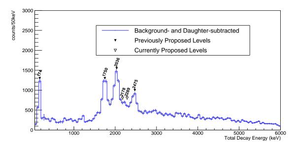
Figure B.4: Final, background- and daughter-subtracted TAS for the <sup>57</sup>Ti decay. Note the two levels from <sup>57</sup>V are now removed. Closed triangles show the previously proposed levels [18], while the open triangles indicate proposed levels from this work.
