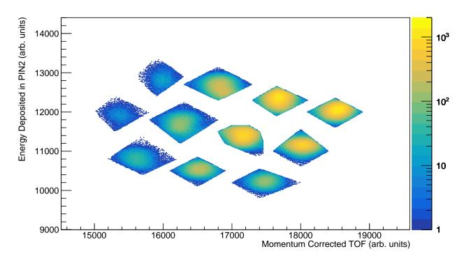
Figure 4.17: Particle ID ( $\delta$ E-TOF) plots for the SuN portion, cut on isotopes of interest. From left to right, top to bottom:  $^{62}$ V,  $^{61}$ V,  $^{60}$ V,  $^{59}$ V,  $^{60}$ Ti,  $^{59}$ Ti,  $^{58}$ Ti,  $^{57}$ Ti,  $^{57}$ Sc,  $^{56}$ Sc,  $^{55}$ Sc.
